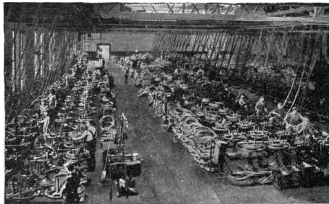
Wire Cut and Shaped by Belt-Driven Machines
